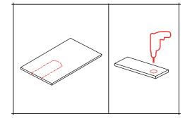
Measure the back of the pan and cut a suitable slot on the main panel to allow for the soil pipe and inlet pipe.
