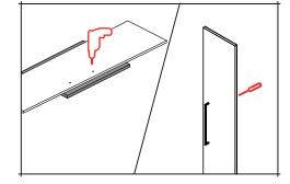
Assemble the door to the carcass and tighten the screws on the hinges ensuring the door is correctly aligned with the carcass.
